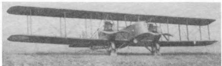
Martin Bomber with two Supercharged Liberty Engines Holds World Records for Two Engined Planes
