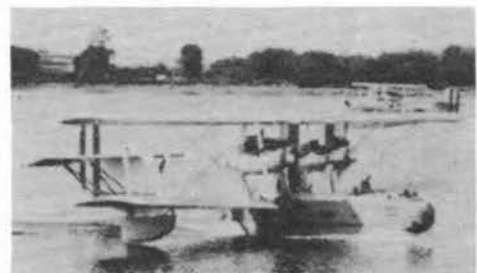
PN-7 Navy Patrol Plane, Speed 100 m.p.h., Equipped with two 525 h.p. Wright Engines
