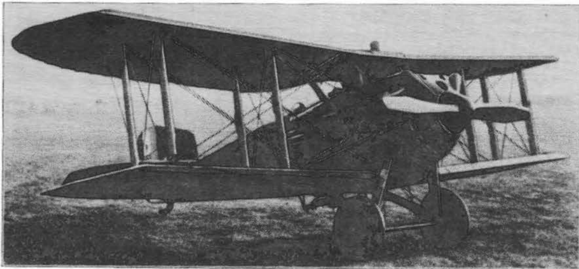
Thomas-Morse MB-3 Pursuit, Equipped with Wright 3A Engine
