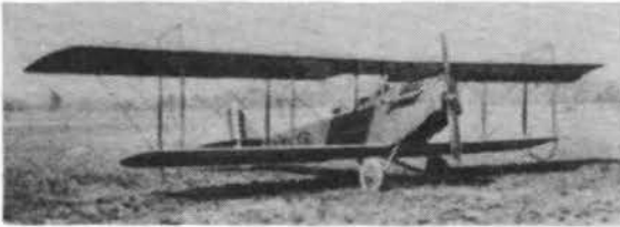
Curtiss "JN" Army Training Plane. Using Curtiss 90 h.p. Engine
