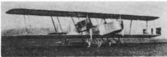
Glenn L. Martin Bomber with Two 400 h.p. Liberty Engines
