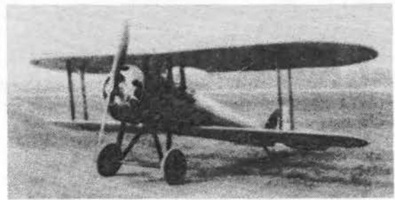
"Nieuport 28" French War Plane with 9 cyl. 140 h.p. Gnome Engine
